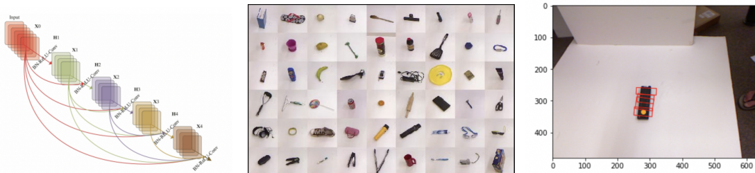
Fig. 1 The architecture of DenseNet. Fig. 2 & 3 Cornell Grasping Dataset with labeled grasps rectangle boxes.
